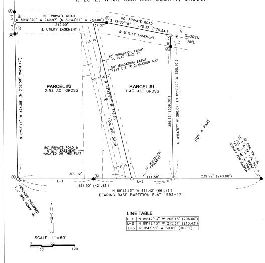
FOUND IRON REBAR ( 1/2" P. PLAT 1990-16 ( 5/8" P. PLAT 1993-17 O SET 5/8"X30" IRON REBAR WITH PLASTIC CAP #951
