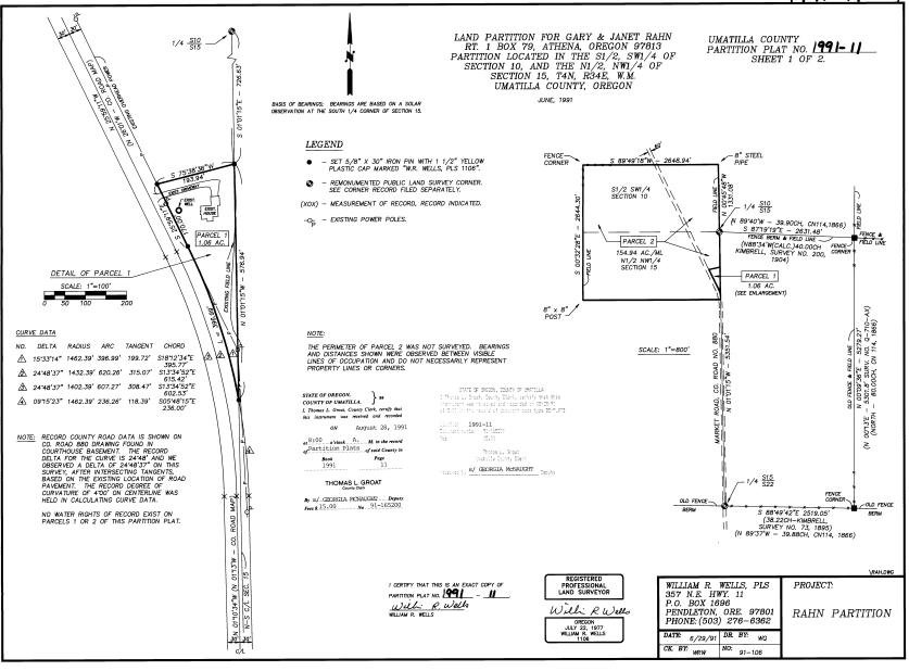
LAND PARTITION FOR GARY & JANET RAHN RT. 1 BOX 79, ATHENA, OREGON 97813 PARTITION LOCATED IN THE S1/2, SW1/4 OF SECTION 10, AND THE N1/2, NW1/4 OF SECTION 15, T4N, R34E, W.M., UMATILLA COUNTY, OREGON
