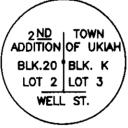
Found corner set by Perry (CS S-8-B) which is a  $2 \frac{1}{2}$  diameter brass cap, set flush with the ground, marked as
