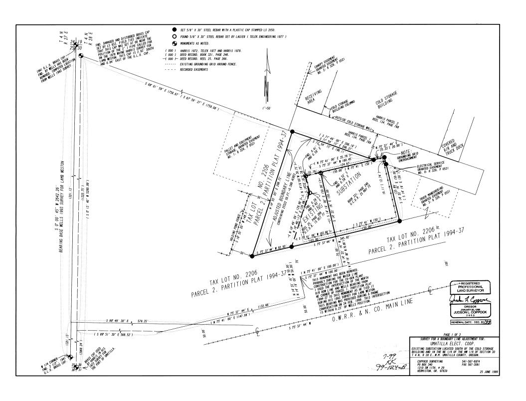
THE PURPOSE OF THIS SURVEY IS TO LOCATE. DESCRIBE AND MONUMENT A TRACT OF LAND LOCATED IN PARCEL 2. UMATILLA COUNTY PARTITION PLAT NO. 1994-37. THIS IS BEING DONE AS A PART OF A BOUNDARY LINE ADJUSTMENT WHICH WILL INCREASE THE AREA OF THAT TRACT OF LAND DESCRIBED IN REEL 25. PAGE 266. UMATILLA COUNTY DEED RECORDS AND OWNED BY UMATILLA ELECTRIC COOPERATIVE.
