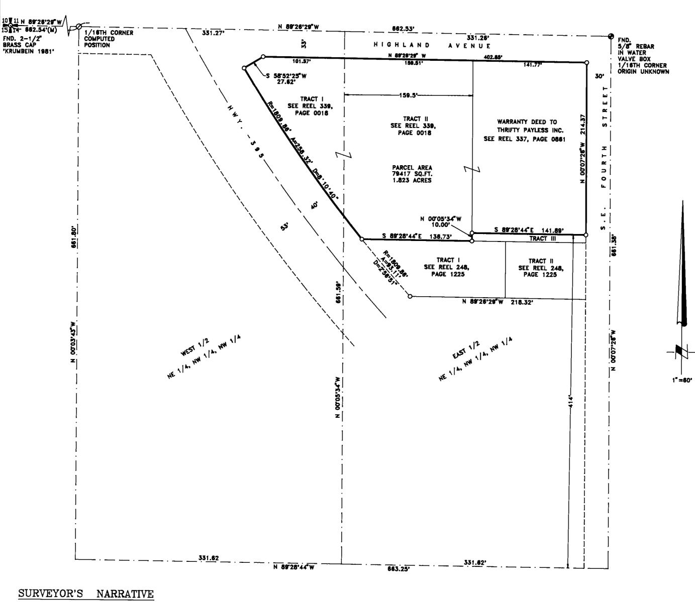
THE PURPOSE OF THIS SURVEY WAS TO MONUMENT THE CORNERS OF THE PROPERTY DESCRIBED HEREON. THE BEARING BASE IS THE NORTH LINE OF THE NORTHWEST QUARTER OF SECTION 14 AS SHOWN ON SURVEY NO. 97-171-B.
