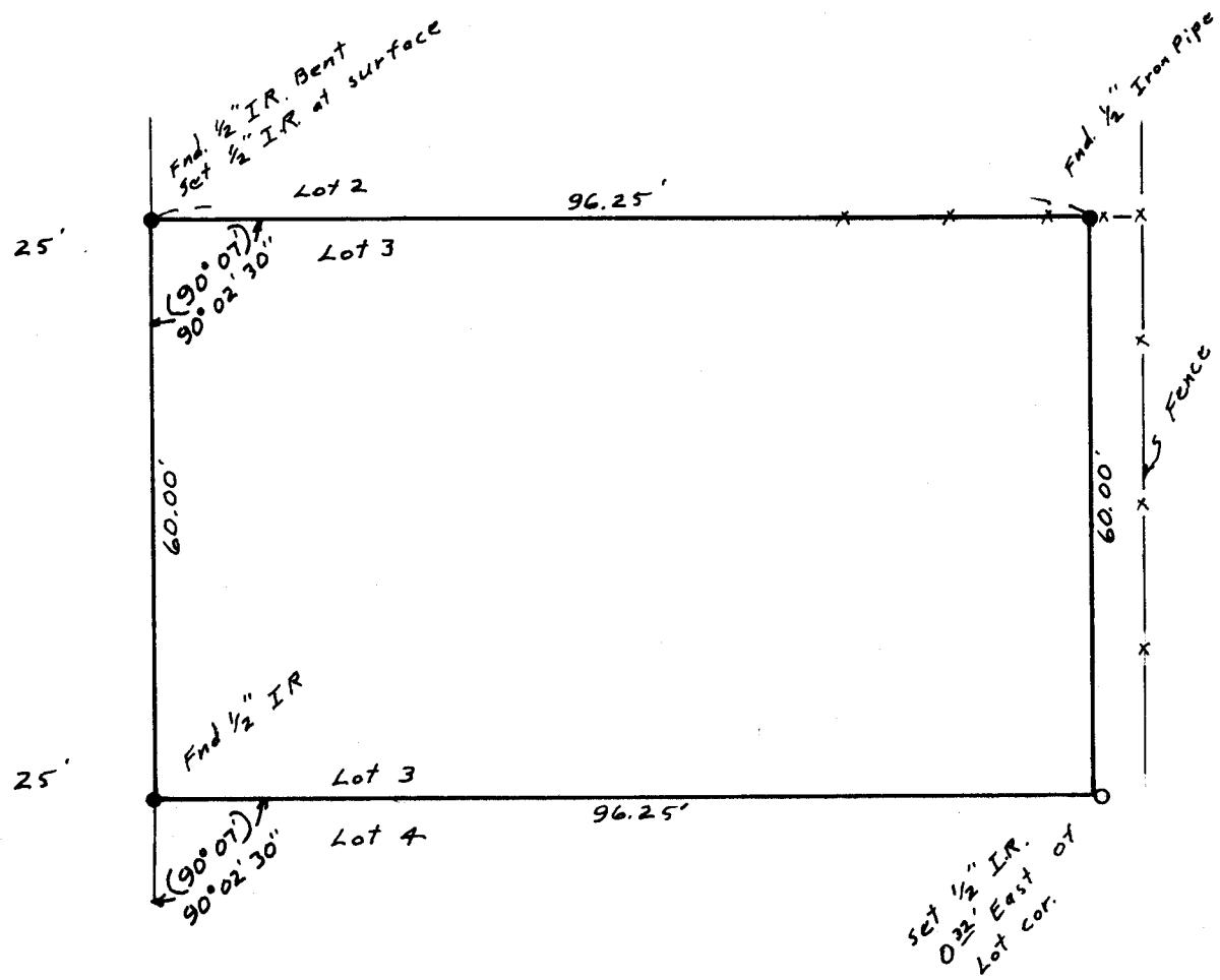
The purpose of this survey is to stake the south line of Lot 3 for the construction of a concrete retaining wall. The found iron rods are probably original corners of "Vickers Add" set in 1851 & the found iron pipe is probably from a more recent survey
