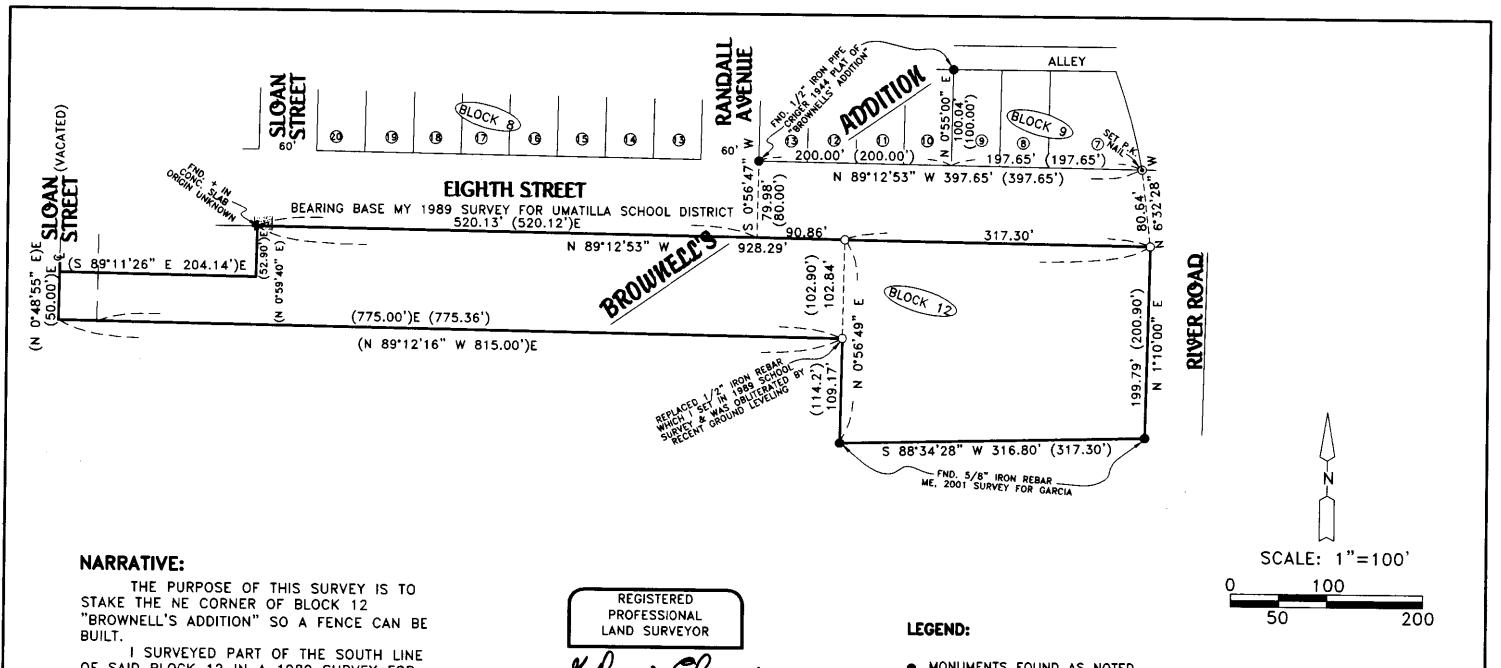
I SURVEYED PART OF THE SOUTH LINE OF SAID BLOCK 12 IN A 1989 SURVEY FOR THE UMATILLA SCHOOL DISTRICT AND ALSO SURVEYED THE WESTERLY PORTION OF THE SOUTH LINE IN A 2001 SURVEY FOR GARCIA AND GROW. I ESTABLISHED THE NE CORNER OF BLOCK 12 BY RETRACING CRIGER'S 1944 SURVEY OF SAID "BROWNELL'S ADDITION".
