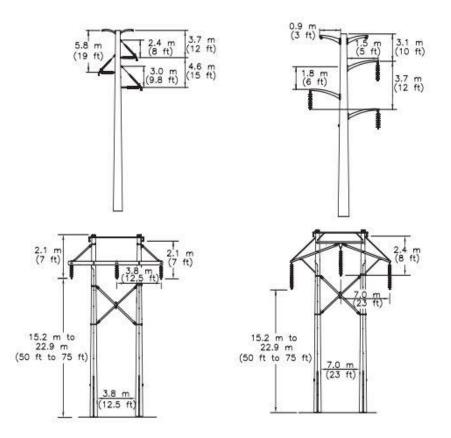
Figure 2. Typical Transmission Structures
