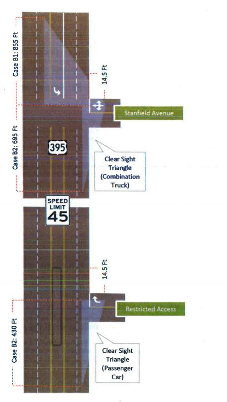
Figure 5. Intersection Sight Triangle Measurements for Case B1 (Left-Turn from Stop) and Case B2 (Right-Turn from Stop) at the right-in, right-out (left) and Stanfield Avenue access (right) connections identified in the IAMP.
